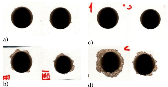
Fig. 1. a) Input holes drilled by undamaged drill, b) input holes drilled by warned out drill, c) output holes drilled by undamaged drill, d) output holes drilled by worned out drill.
