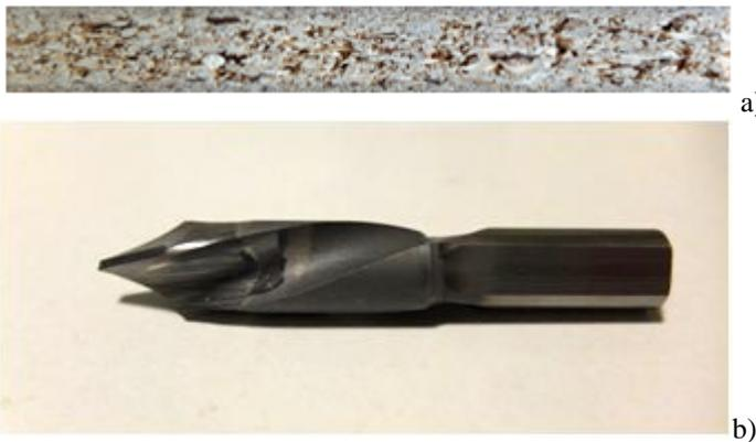
Fig. 2. The image of a) laminated chipboard, b) drill used in experiments.
