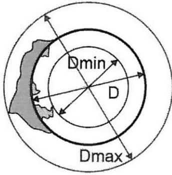
Fig. 4. Interpretation of diameters used in generating numerical features.
