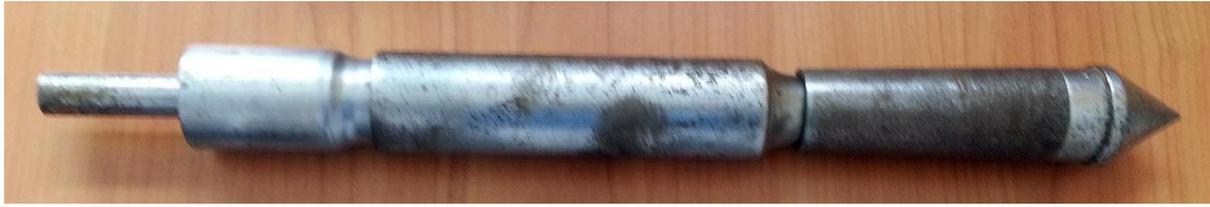
**Figure 1 The cone penetration test probe**
