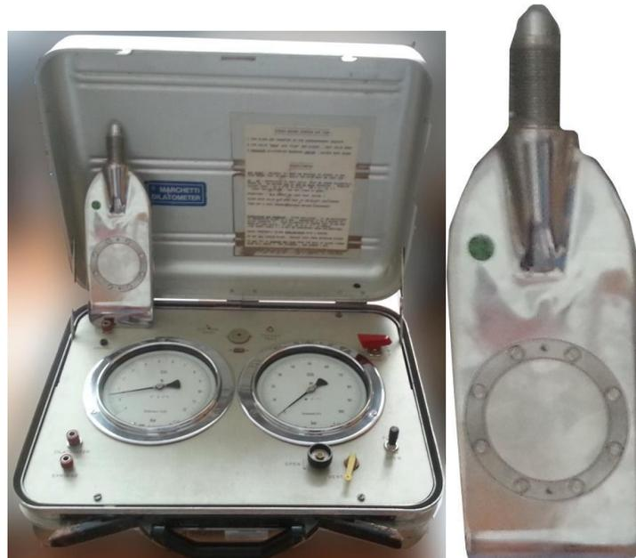
**Figure 2 The DMT control unit (left) and the probe (right)**
