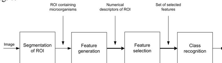
FIGURE 1. The proposed system of recognition of the microorganism classes.
