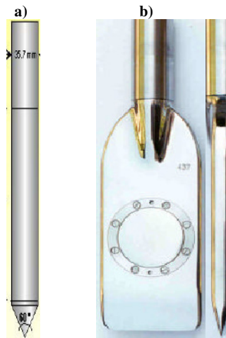
Figure 1 View of CPTU tip (Mayne et al., 1995) (a) and DMT blade (b) used in the situ tests
