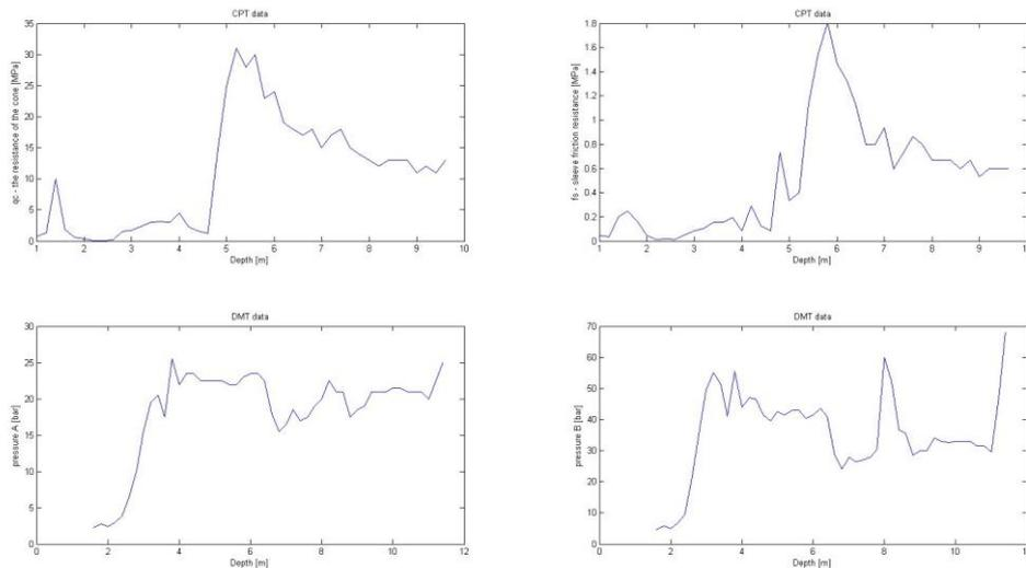
Figure 4. Results of the CPT and DMT measurements
