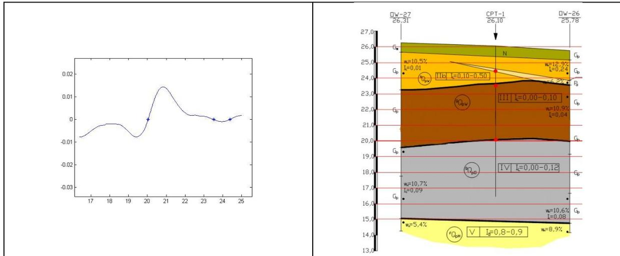
Figure 6. Results of the CPT measurements a) result of cubic interpolation b) Gaussian filtering c) Gaussian filtering and its derivative (blue line ) d) first derivative and its zero crossing e) geotechnical cross-section
