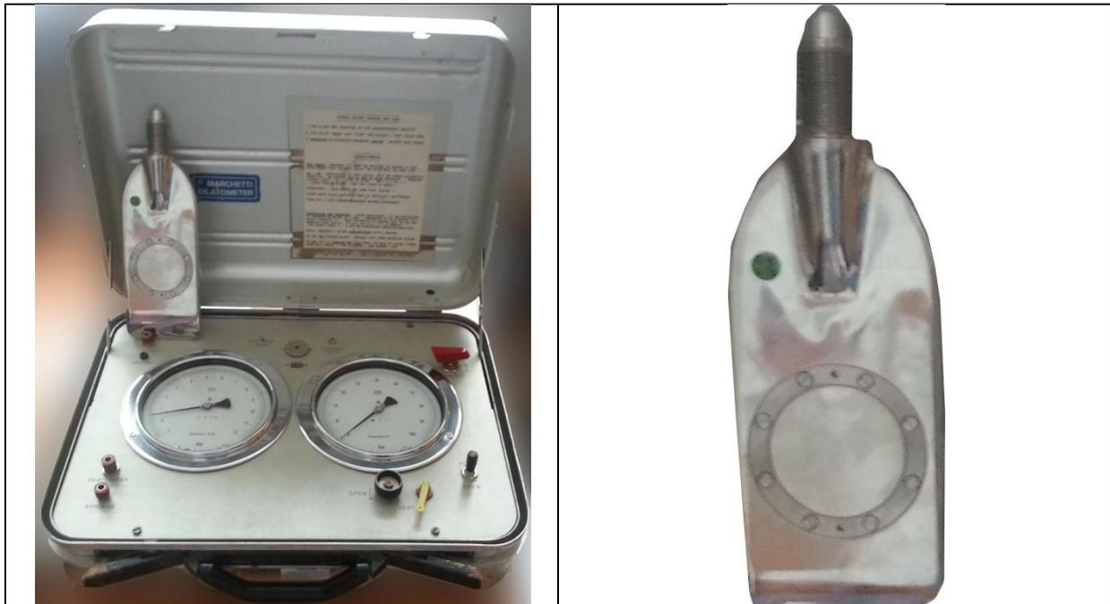
Figure 2 : The DMT control unit (a) and the probe (b)
