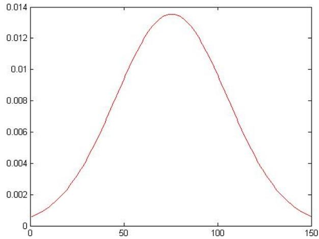
Figure 5. The Gaussian window
