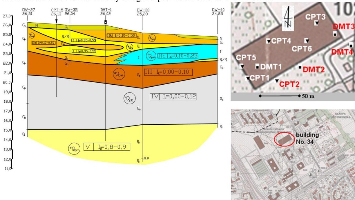
Figure 3. A typical geotechnical cross-section: OW – borehole, CPT – cone penetration test, DMT – Dilatometer test; (N – fill, Gp – sandy clay, Pd –fine sand,  $w_n$  – moisture content,  $I_D$  – relative density,  $I_L$  –liquidity index)
