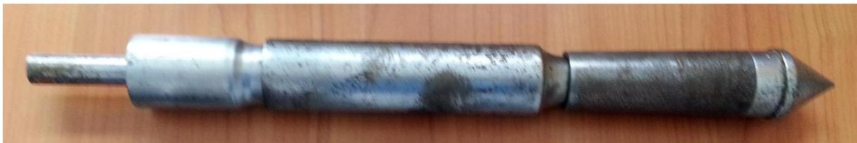
Figure 1 : The cone penetration test probe
