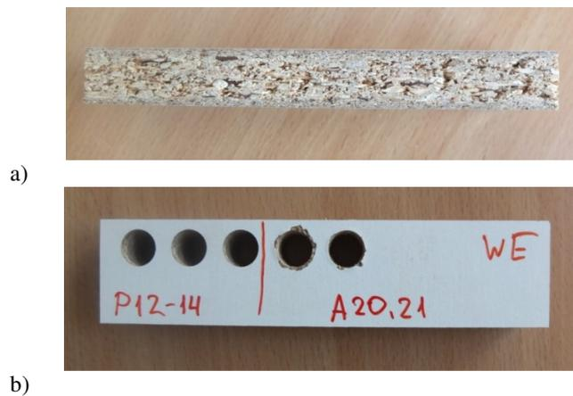
Figure 3. Standard laminated chipboard used in experiments (a) and view on examples of five drilled holes (b).
